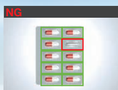
① Missing Pill
